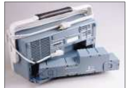
TDS 3BAT – Battery Pack being installed.
